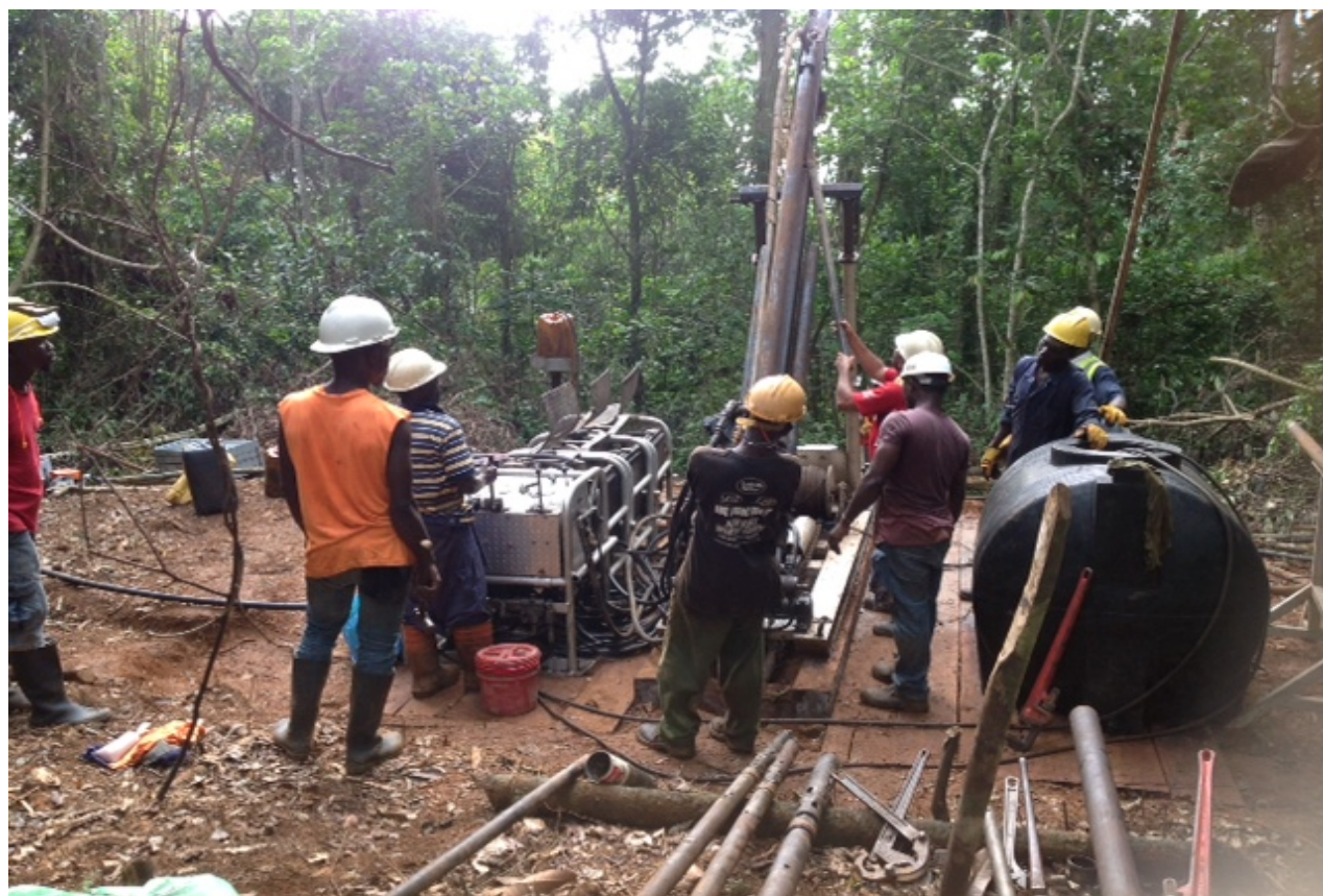
Figure 4 | Diamond Core drill rig being set up at Goehn SE Deposit
