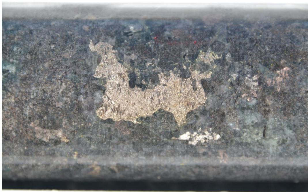
FIGURE 2: Core from MRDD011 showing blebby sulphides at depth 211.20 metres. Portable handheld Niton XRF readings range from 1.9% up to 3.9% nickel and from 0.1% up to 1.7% copper.
