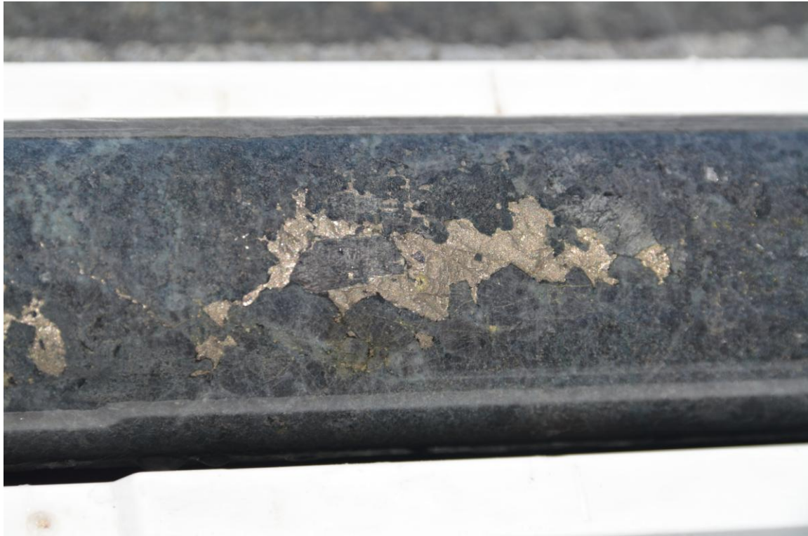
FIGURE 3: Core from MRDD011 showing large sulphide bleb at depth 337.60m. Portable handheld Niton XRF readings range from 1.2% up to 2.9% nickel and from 0.4% up to 0.7% copper.
