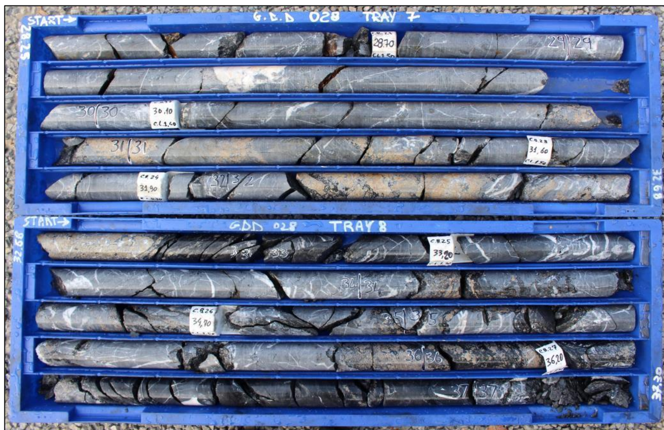
Figure 2 – Massive and disseminated zinc sulphides in GDD028
