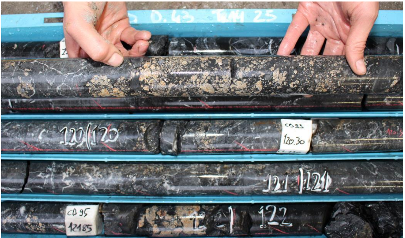
Figure 3 – Semi massive and disseminated zinc sulphides in GDD043
