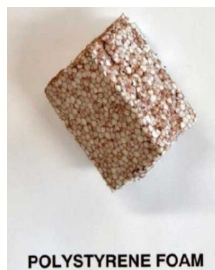
Figure 4: Flame retardant insulation foam
