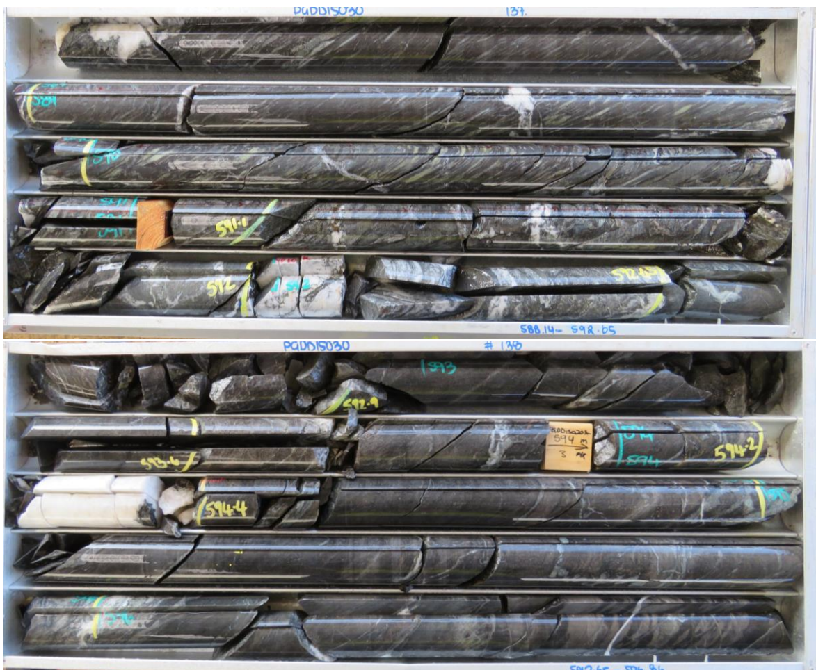
Figure 4 - PGDD15030 K2 laminated quartz vein on the sheared contact of the Victorious basalt and volcanoclastics.
