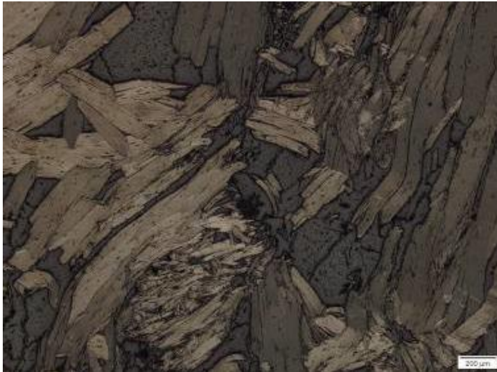
Figure 1: In-situ graphite flakes approximately 0.4 to 1mm long (400 \mu m-1,000 \mu m) associated with coarse-grained quartz
