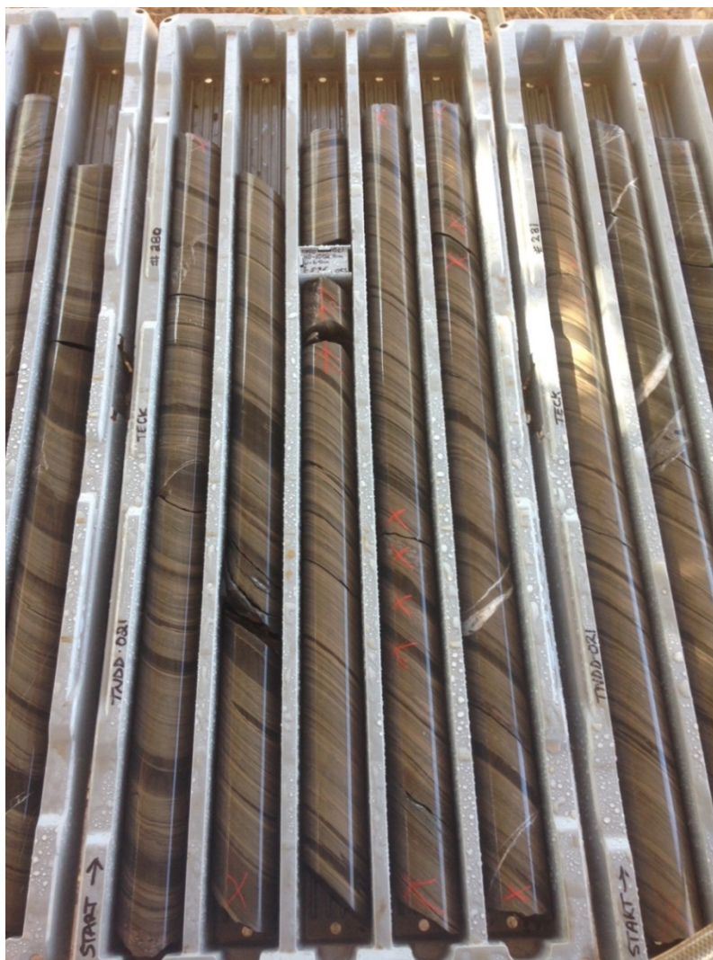
Figure 4: Mineralised core from hole TNDD021. The creamy brown mineral is sphalerite (zinc sulphide)
