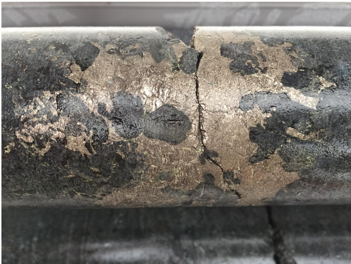
FIGURE 2: Core from MRDD010 showing stringer sulphides at depth 179m. Note the sulphides encasing large olivine and pyroxene crystals.
