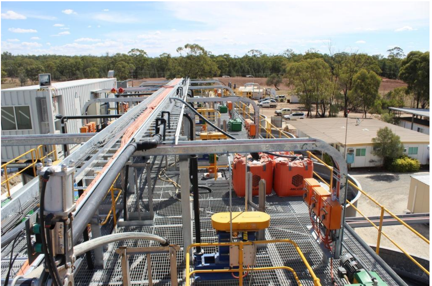
Photograph 1. Carbon bulka bags ready for addition to the CIL circuit.
