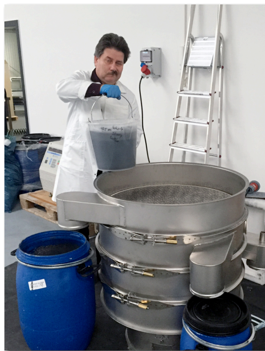
Figure 4. Phase 1 samples being sieved in new equipment at Rudolstadt test facility.
