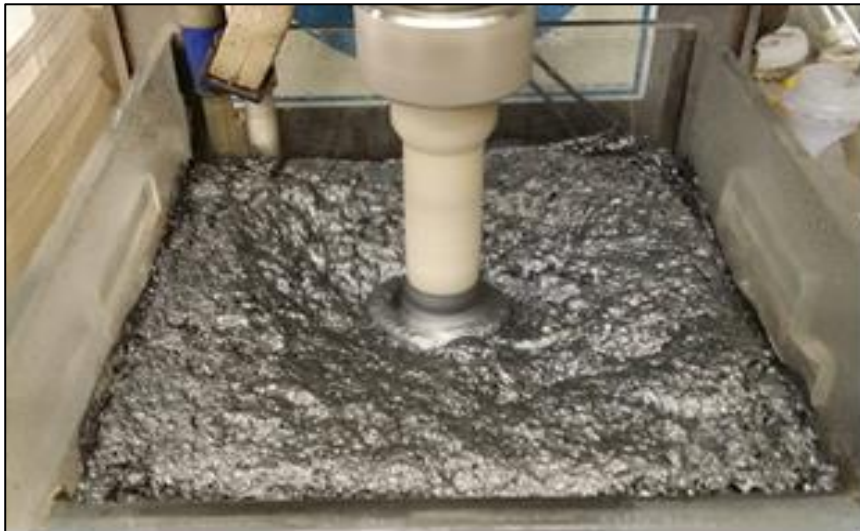
Image 1: Lindi Jumbo concentrate being float tested
