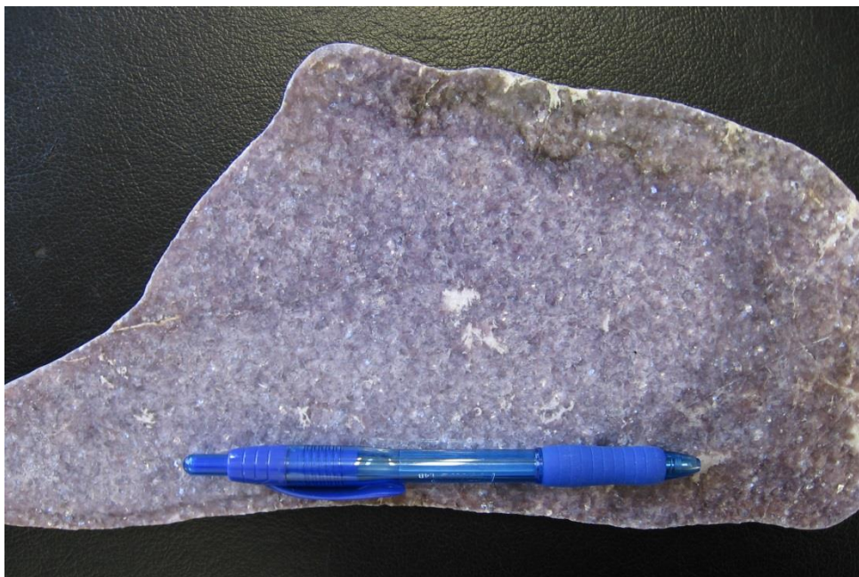
Figure 1: Photo of a polished rock specimen containing high-grade lithium from the Mt Alexander Project (purple coloured mineral is the lithium rich mica – lepidolite)
