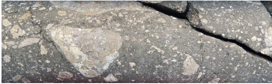
Figure 1a: LEFT core photo at 256.2m showing matrix supported tourmaline breccia with arsenopyrite / pyrite replacement of clasts and matrix. The metre sample grade is 1,995g/t Ag, 2.22g/t Au, 0.86% Cu and 2.7% Pb.
