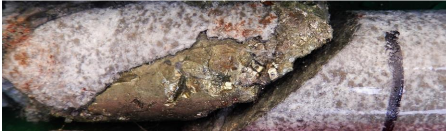
Figure 1b: LEFT core photo at 792.95m showing chalcopyrite vein cutting through porphyry. The metre sample grade is 5.80% Cu, 27g/t Ag.
