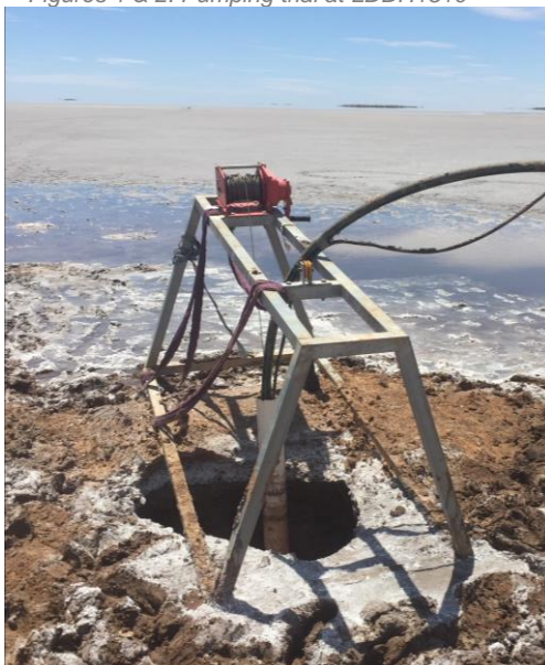
Figures 1 & 2: Pumping trial at LDDH1510
