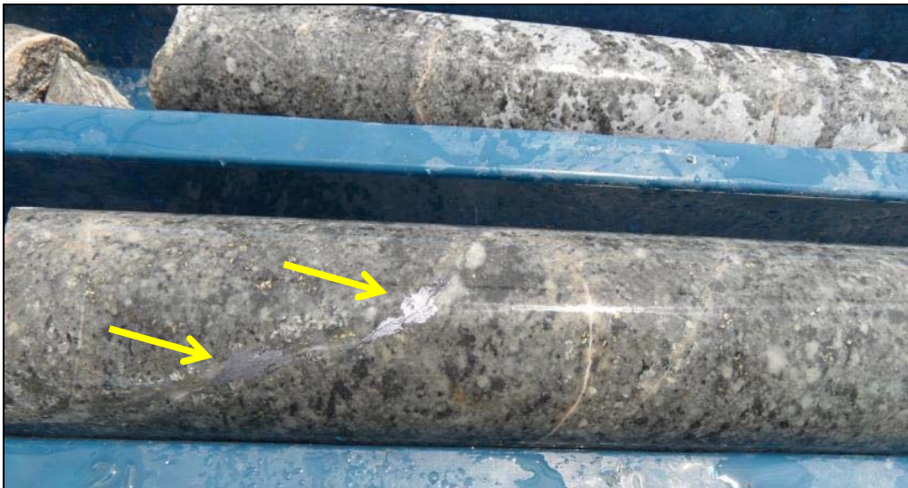
Photo 4: Example of molybdenum veining present at Joshua.
