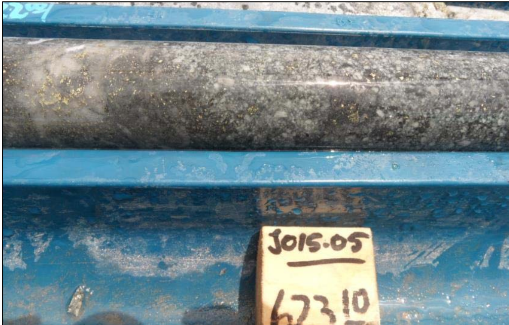
Photo 3: Disseminated Chalcopyrite at 623m in JO-05
