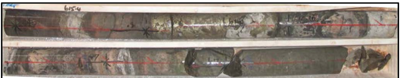
Figure 2: MHC20001 drilled in 2012 (615.80 to 616.16m) Minyari deeps brecciated chalcopyrite-quartz-calcite sulphide vein identical in style to the Telfer mineralisation assemblages (0.36m at 41.55 g/t gold, 12.02% copper and 43.80 g/t silver).
