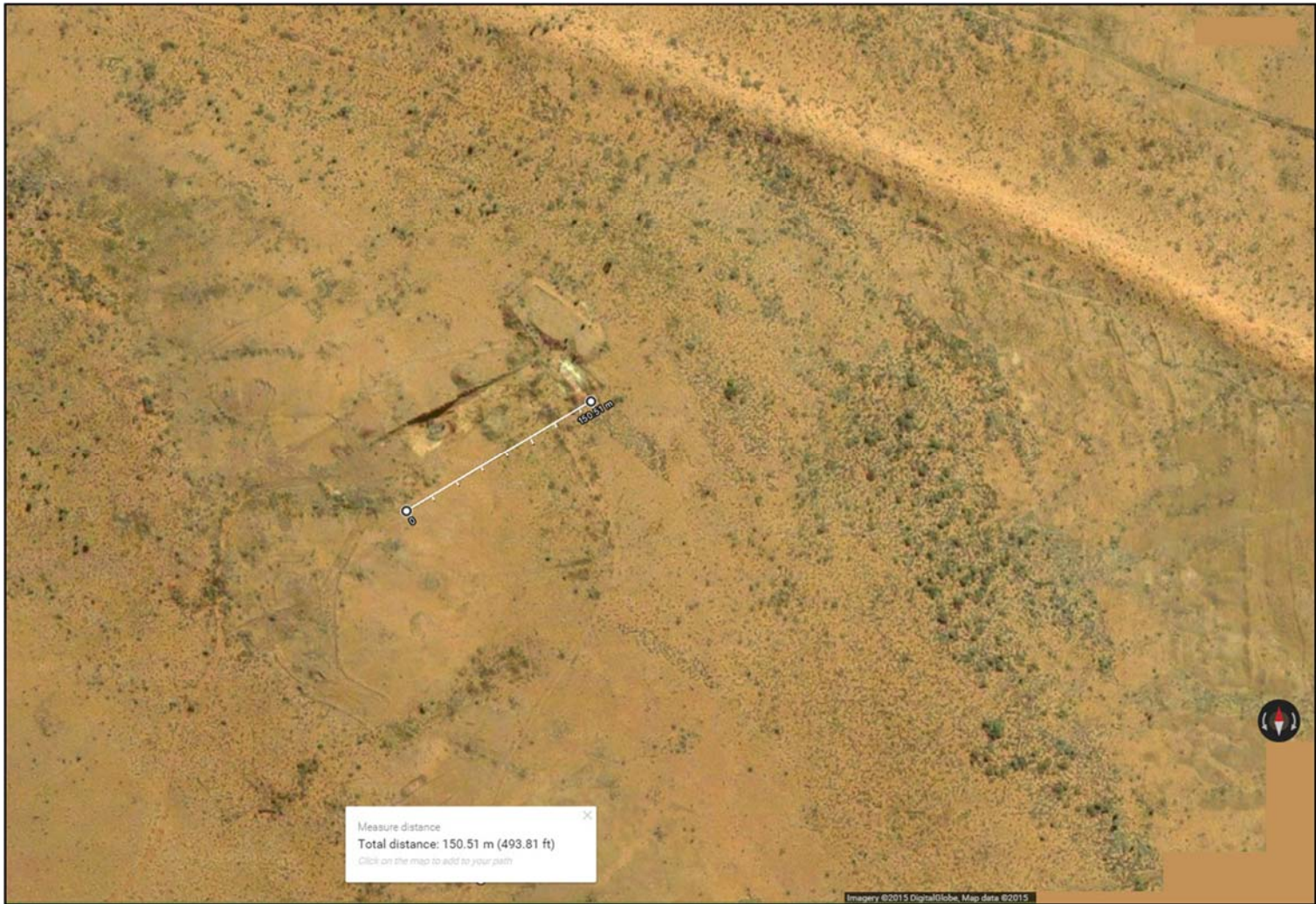
Minyari Deposit costean (150m in length) constructed by Newmont in 1987 for purposes of collecting metallurgical sample material (i.e. 2 x 8 tonnes, i.e. 16 tonnes in total) – Plan (Satellite) view.
