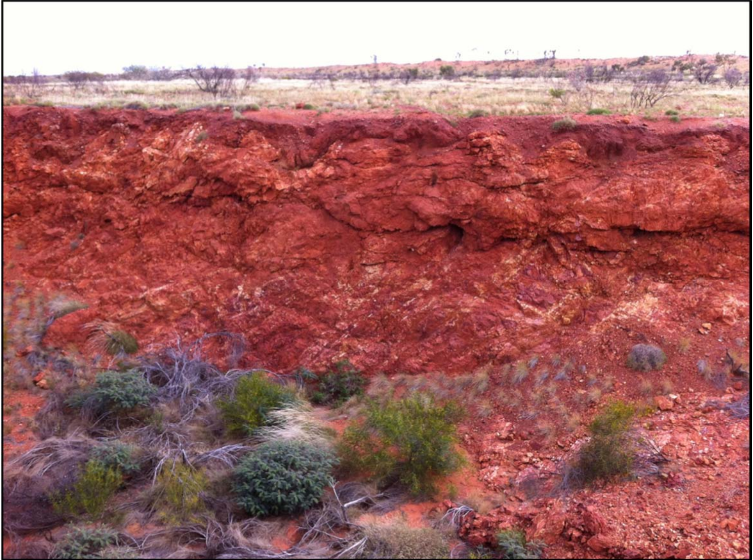
Minyari Deposit southwest dipping oxide gold mineralisation (gossanous quartz veins) under less than 1m of cover exposed within costean (constructed by Newmont in 1987 for purposes of collecting 2 x 8 tonnes, i.e. 16 tonnes of metallurgical sample material) – Looking north.
