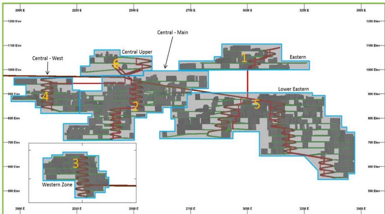
Figure 6: SSO Mining Sequence (long section looking North)
