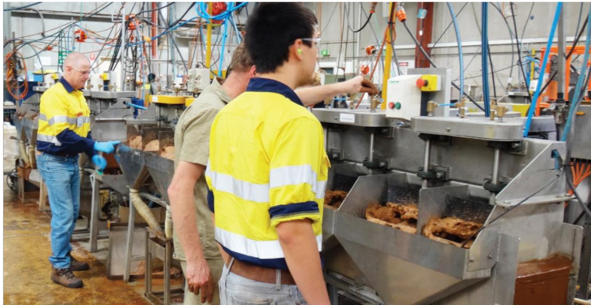
Image: Commissioning of the Barite Prefloat Circuit (2015)
