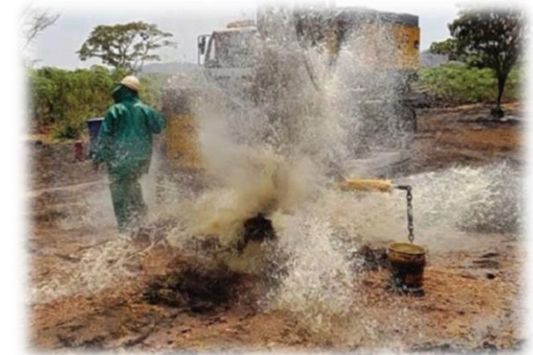
Image: Water intersected ion drill hole MWB008 with flow estimated at over 10L/s, Ngualla, September 2015
