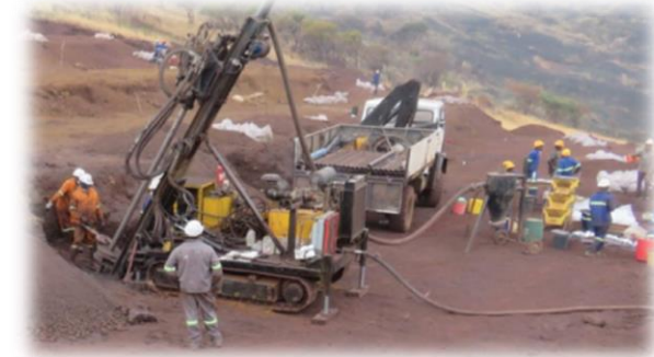
Image: RC drilling on trial grade control grid, Ngualla, August 2015
