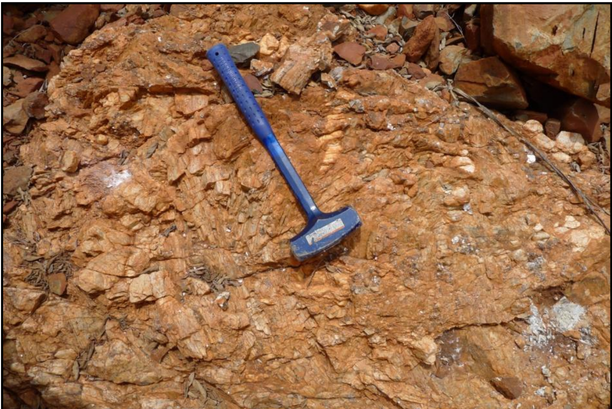
Figure 3: Exposure of the Track Pegmatite showing spodumene crystals up to 20cm long. The outcrop grades 3.86% \text{Li}_2\text{O} and 196ppm Ta.
