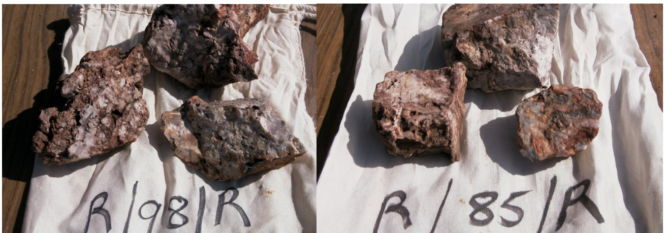
Figure 4: Chalcedonic quartz and minor grey sulphidic silica rock chip sample reporting 422 ppm Au & 360 ppm Ag (sample R/85/R) and 35.1 ppm Au & 13.5 ppm Ag (sample R/98/R).
