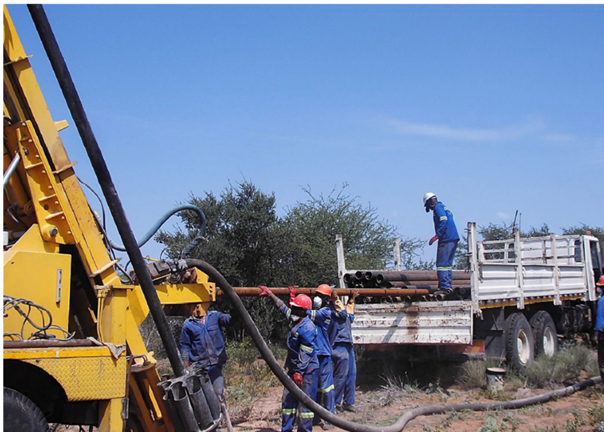
Figure 2: RC drilling in progress at Aphrodite Prospect, T4
