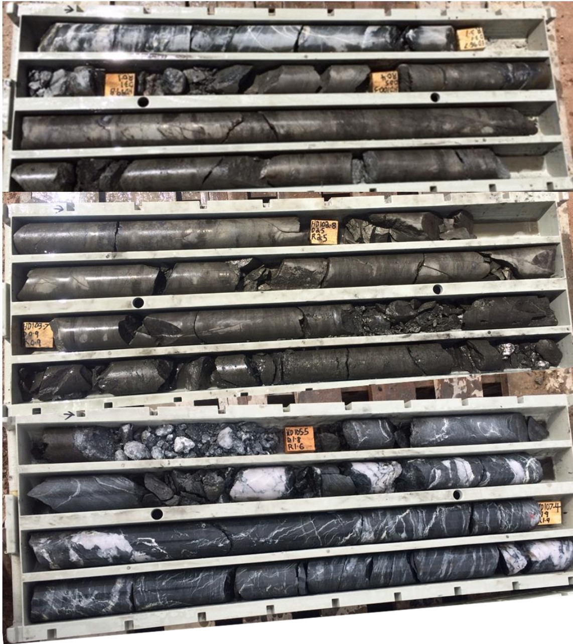
Figure 2: Photos of core from 99.8m in CODD001 illustrating copper mineralisation in massive, semi-massive and vein type mineralisation from 99.8m-105.5m, core photo finishes at 108.5m
