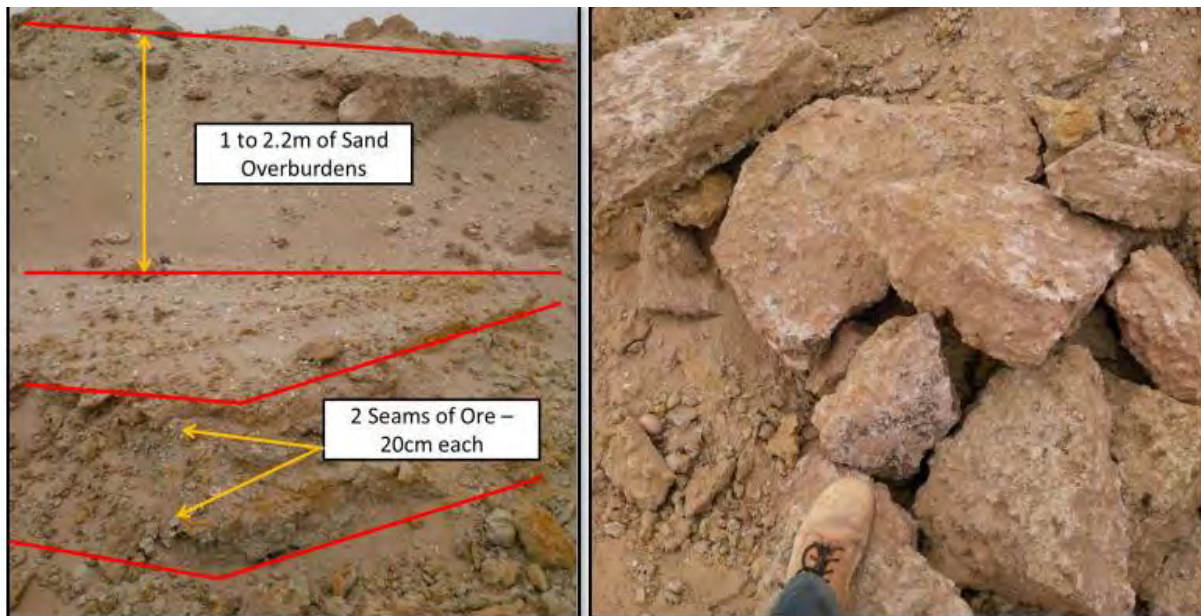
Figure 5:2 Typical Stratigraphic Profile
