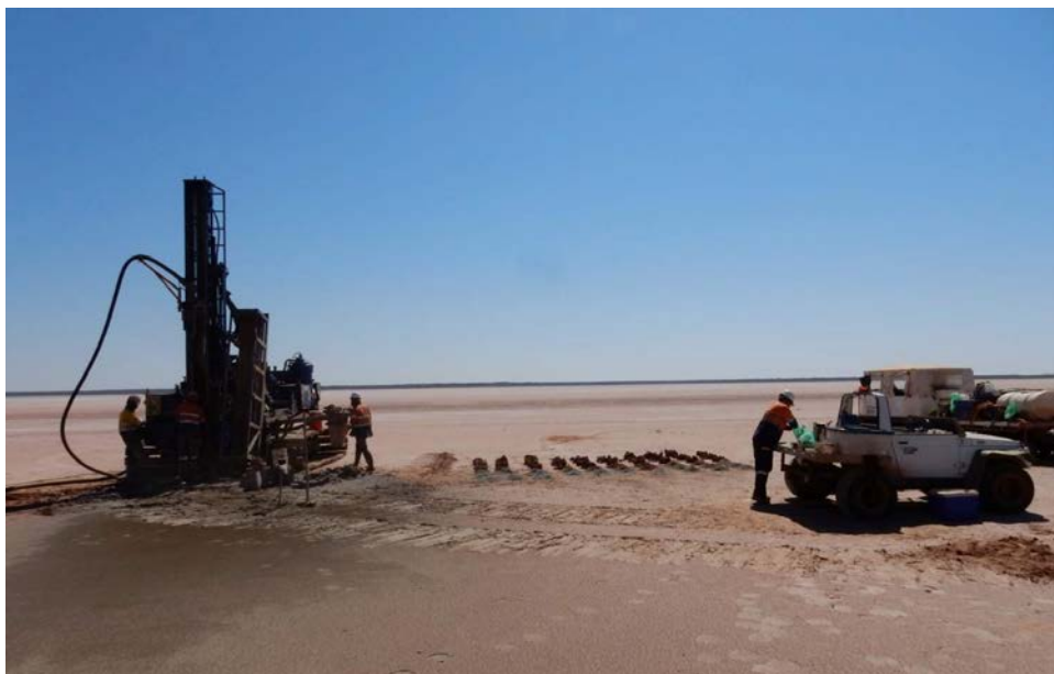
Air Core Drilling in Progress at Lake Wells
