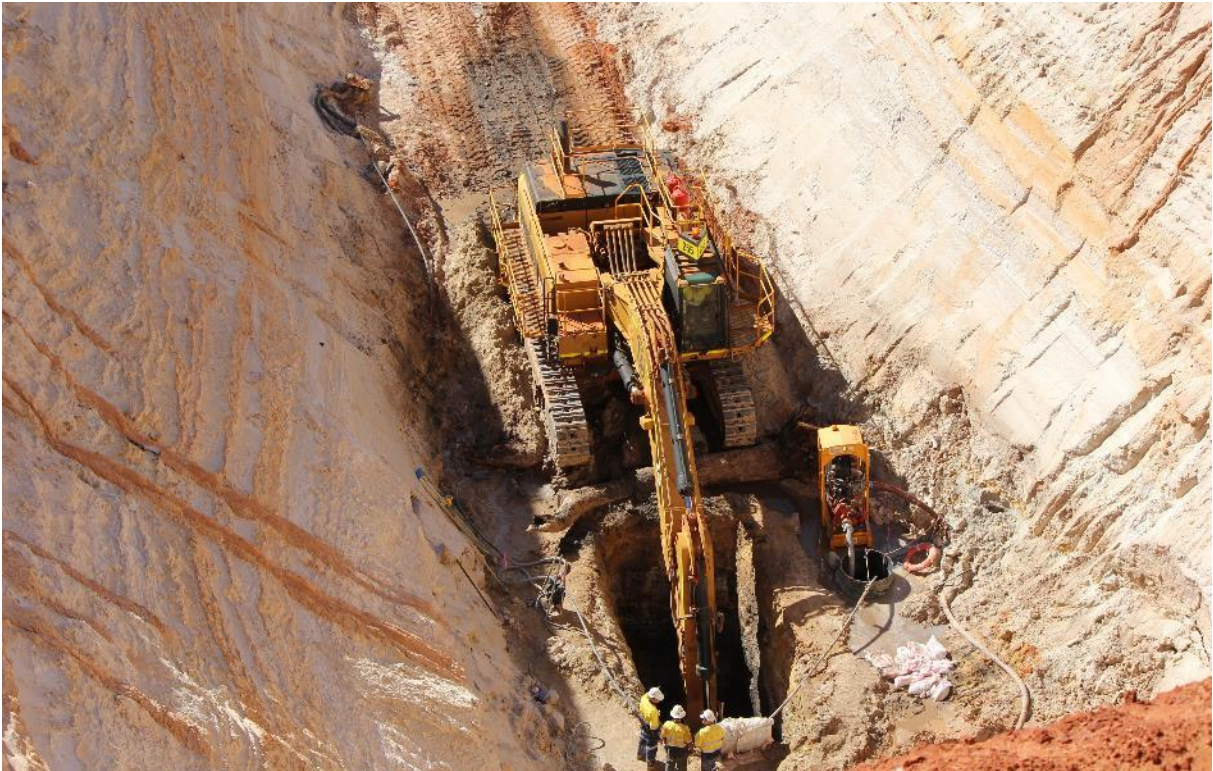
Figure 5: Excavation of bulk ore sample from Ambassador East test pit
