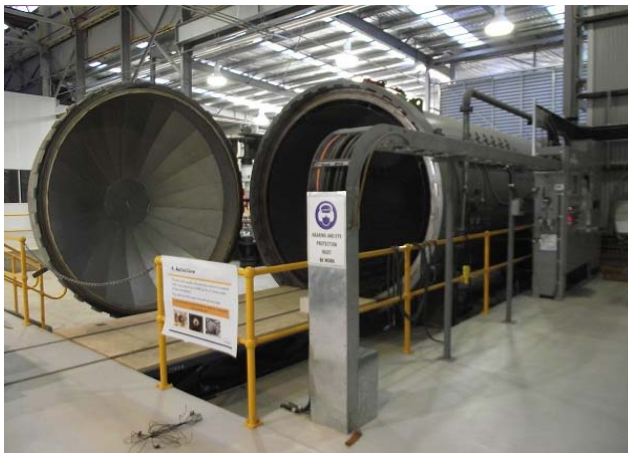
Traditional Autoclave Curing
