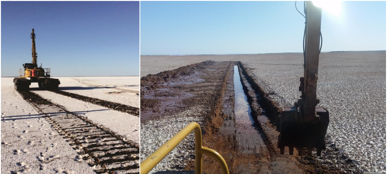
Figures 6 & 7 – Amphibious Excavator Operating on LD
