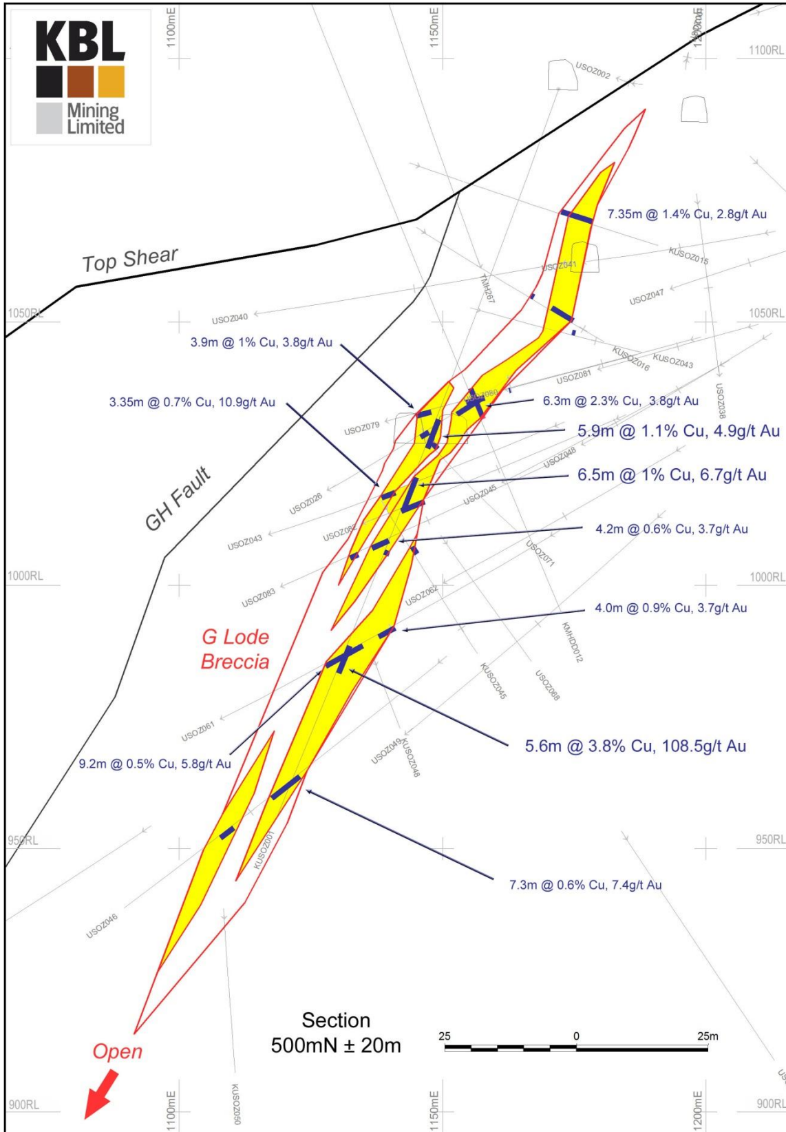
Figure 2. 500N section of G Lode with selected significant historical drill intercepts including those quoted from KUSOZ001. An interpretation of the several mineralised breccia lenses is also presented (yellow)
