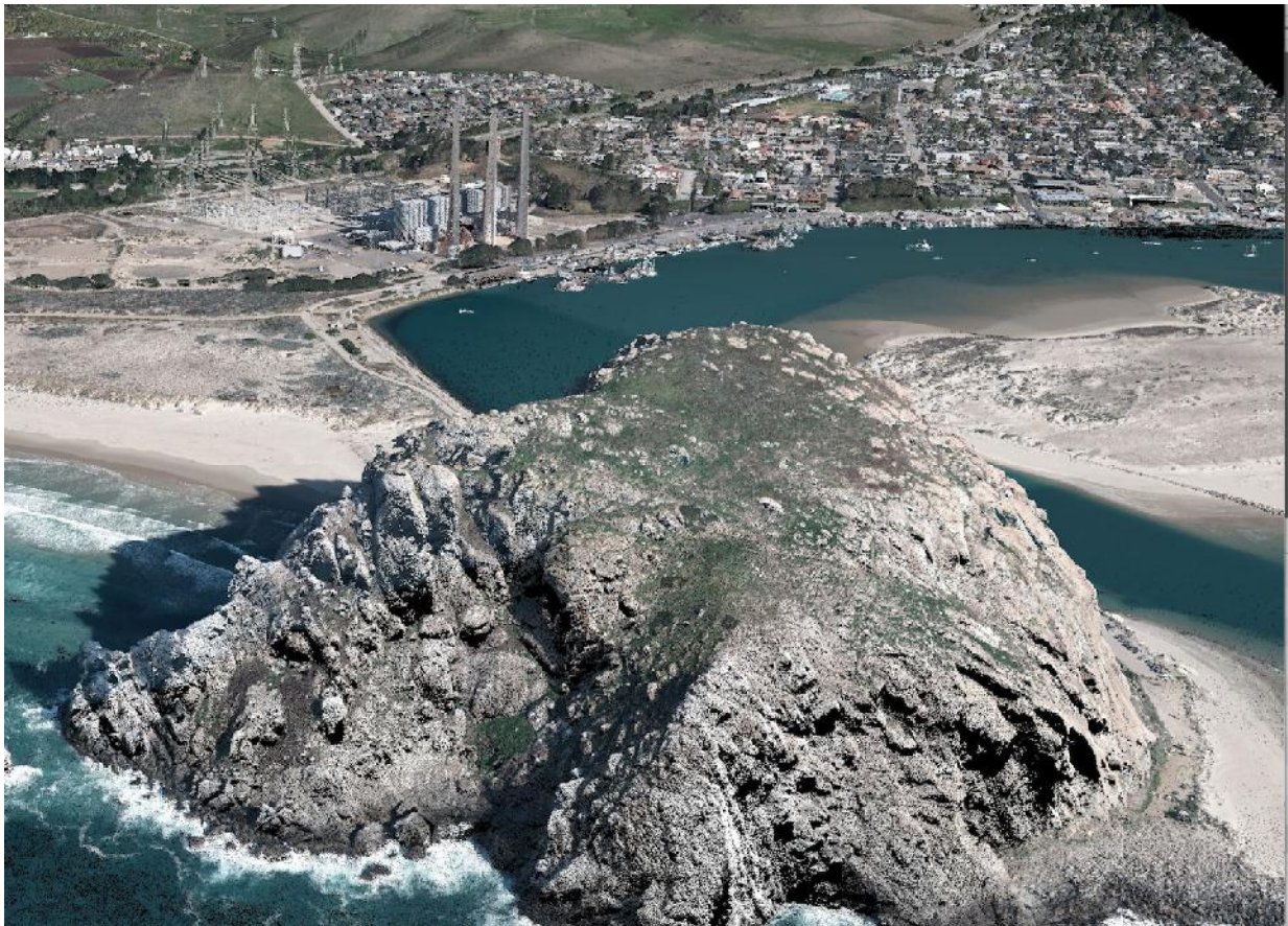
Morro Bay California. Point cloud image taken from a Pointerra processed 25Gb 3D point cloud dataset containing 5 billion points.
