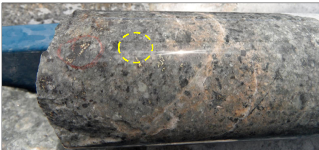
Photo 3: Chalcocite replacing Chalcopyrite in JO-05
