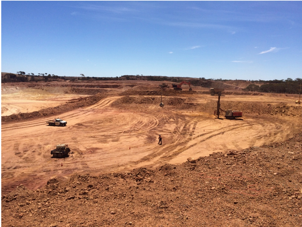
Figure 2 – Early stages of Zoroastrian Central Pit showing drill and blast drilling and waste removal in the southern part of the pit
