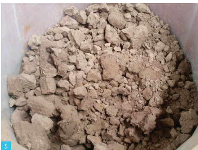
Figure 14: Beneficiation piloting at ALS. 1. Crushed sample prior to primary grinding and Barite Pre-flotation circuit; 2. Crushing Circuit Layout; 3. Barite Pre-flotation Circuit (Roughing stage); 4. Rare Earth Flotation - final concentrate (Cleaner 4 Concentrate); 5. Rare Earth Concentrate grading ~45% REO; 6. Two tonnes of Rare Earth Concentrate ready for delivery to ANSTO.
