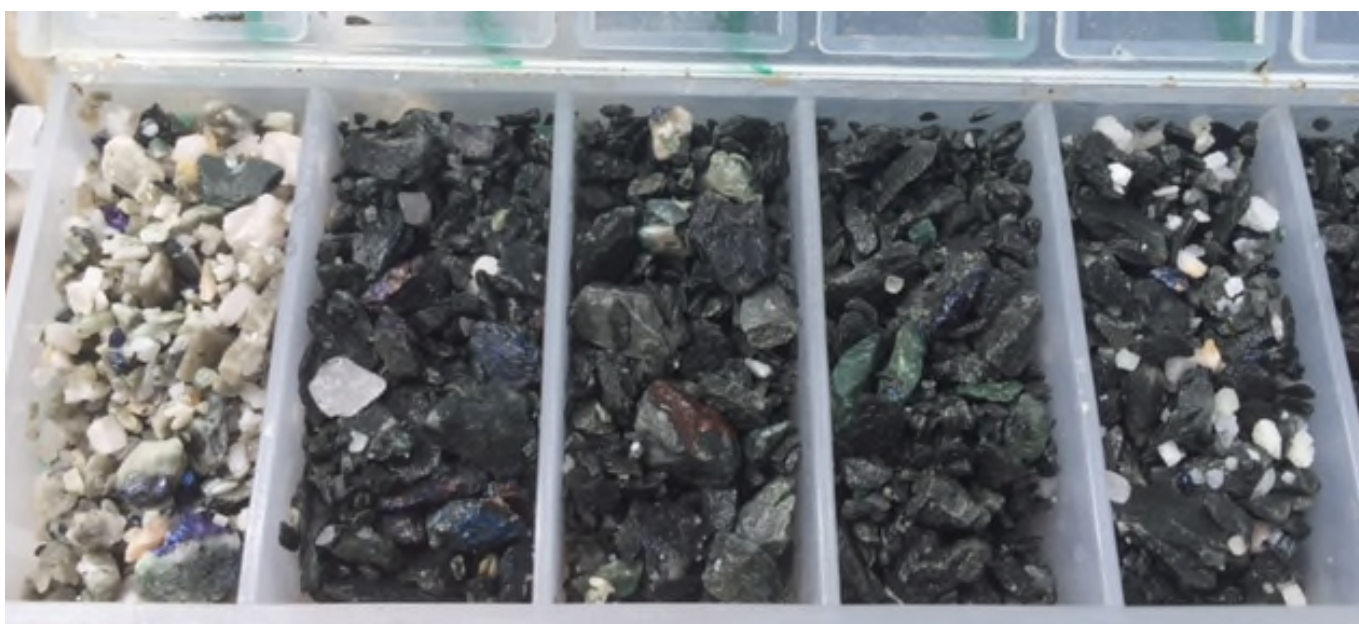
Figure 2: 5m interval in MO-G-12R (120 - 125m) showing vein hosted bornite and chalcopyrite mineralisation
