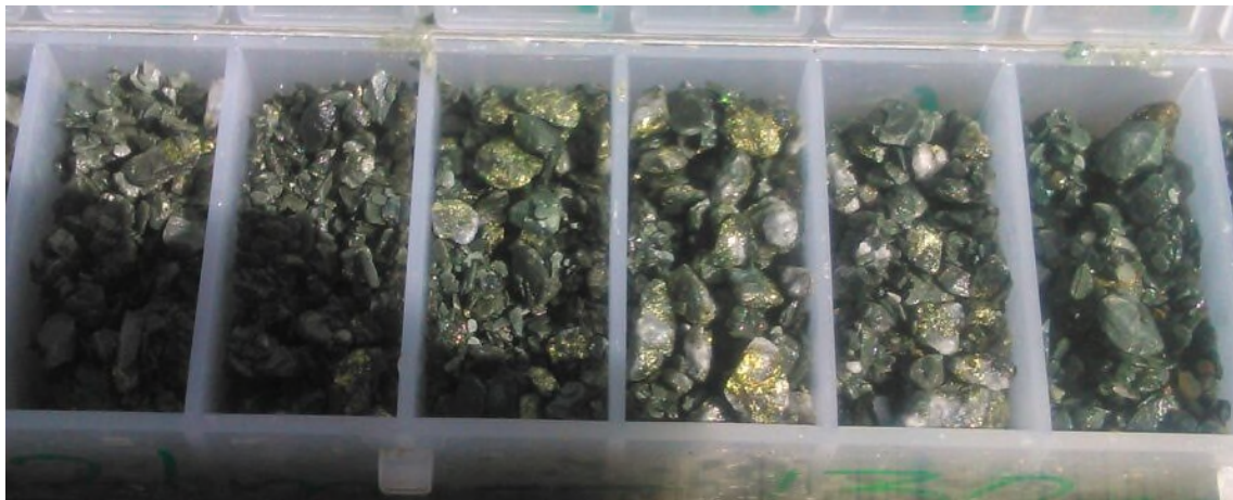
Figure 1: 5m interval in drill hole MO-G-13R (124 -129m) showing quartz vein hosted chalcopyrite mineralisation
