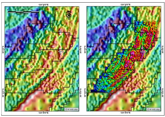
Figure 1: Bouguer 1VD gravity image (Segue 1,600m x 100m on left, MMG 400m x 200m on right)
