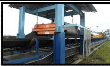
Metal Detector and transfer Conveyor
