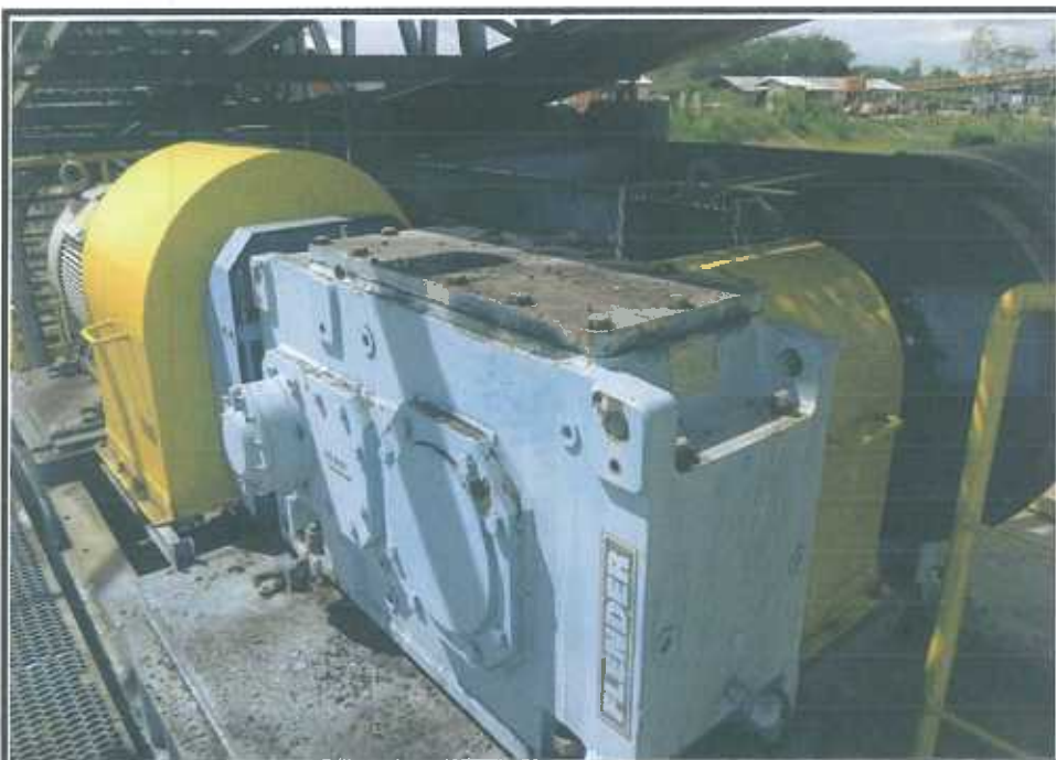
GEAR BOX & ELECTRICAL MOTOR STACKING BELT CONVEYOR
