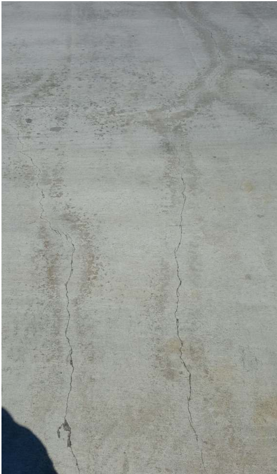
Figure 2. Control slab showing considerable cracking However, the EdenCrete™ enriched concrete trial pad is still in good condition (see Figure 3 )
