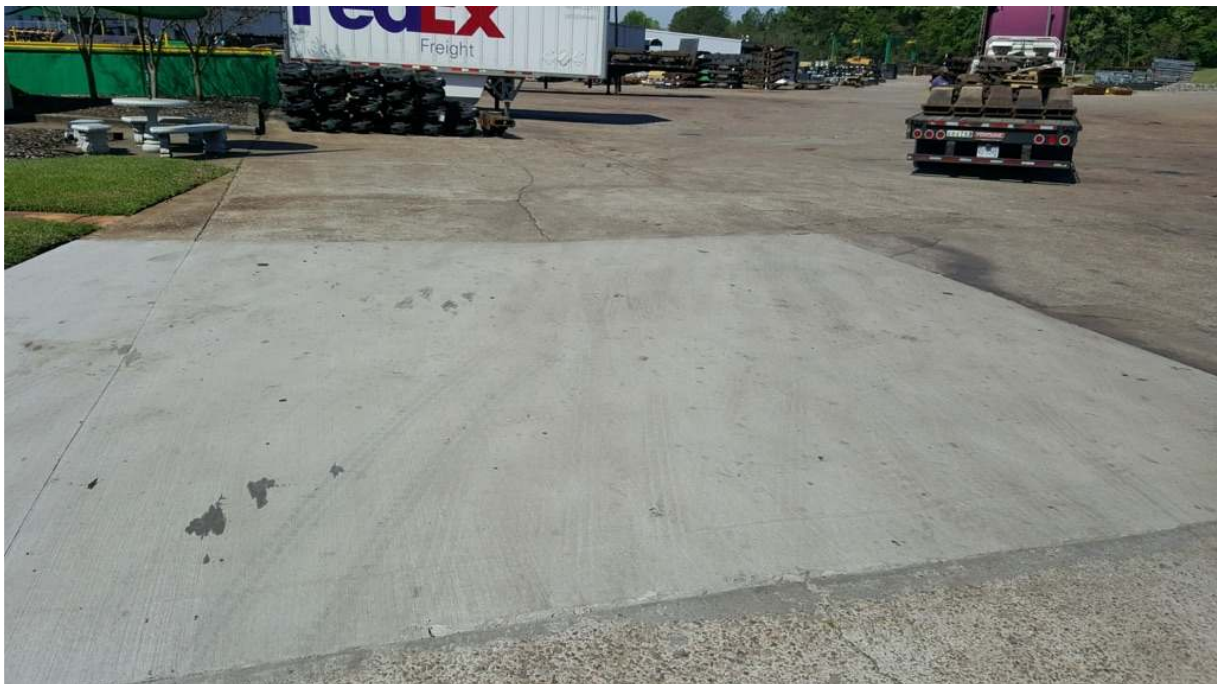
Figure 1. EdenCrete™ field trial slab in foreground with heavily loaded semi-trailer carrying a typical load in upper right of photograph
