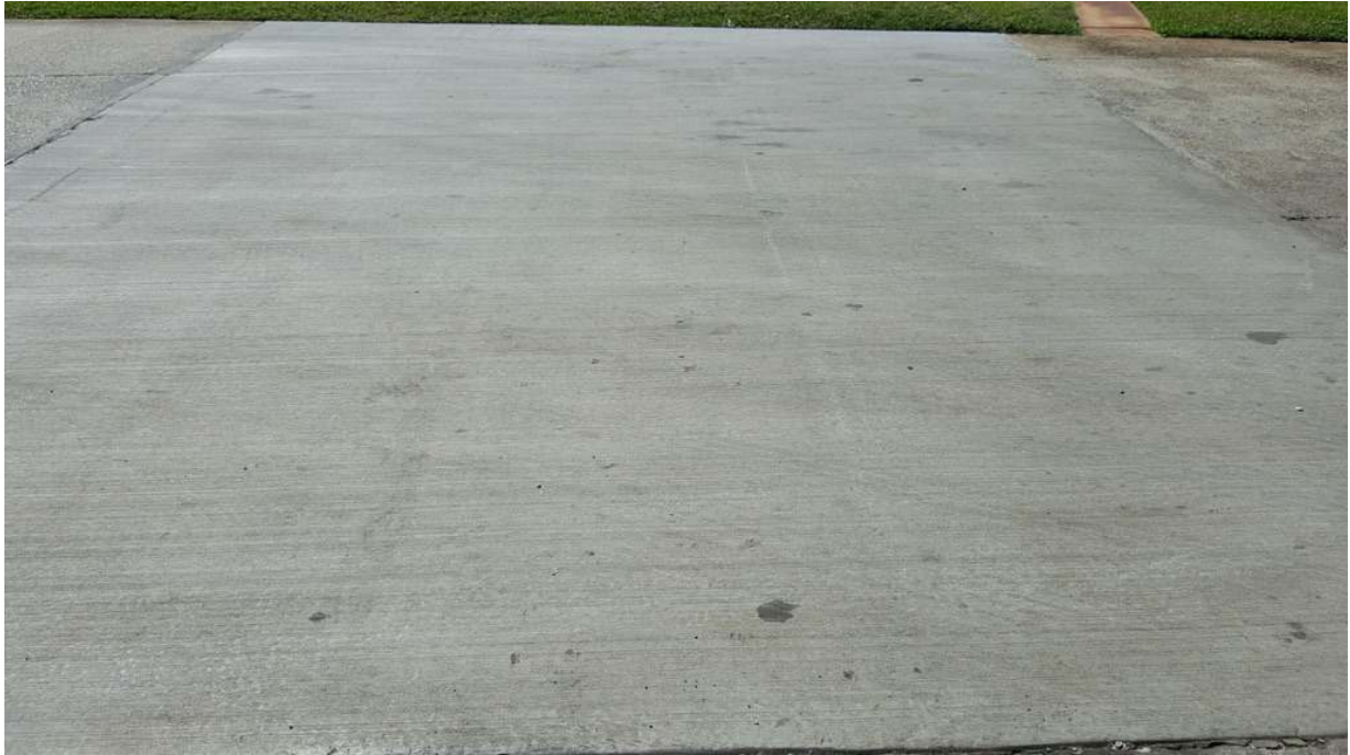
Figure 3. EdenCrete™ Field Trial Slab showing no cracking or damage
