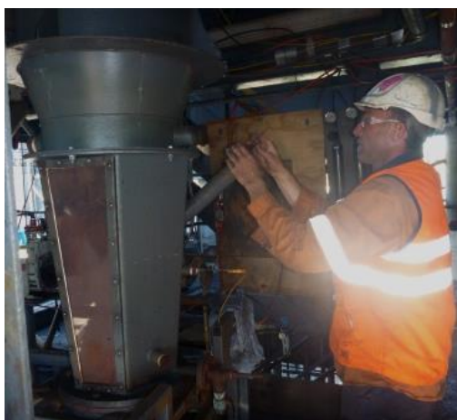
Adjusting the pilot scale fluid bed evaporator during start-up
