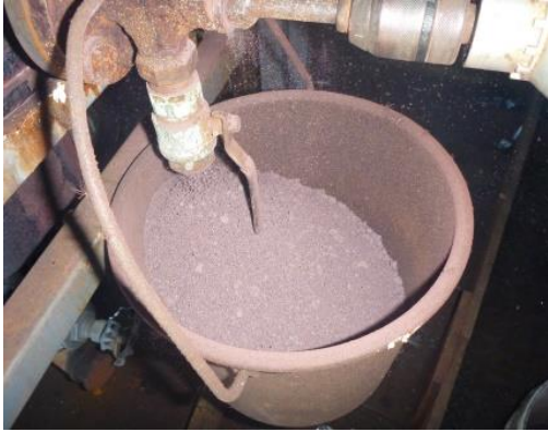
Discharging iron chloride/iron oxide pellets from the fluid bed evaporator (3 rd June)
