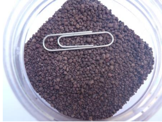
Iron chloride/iron oxide pellets (1-4mm in diameter)
