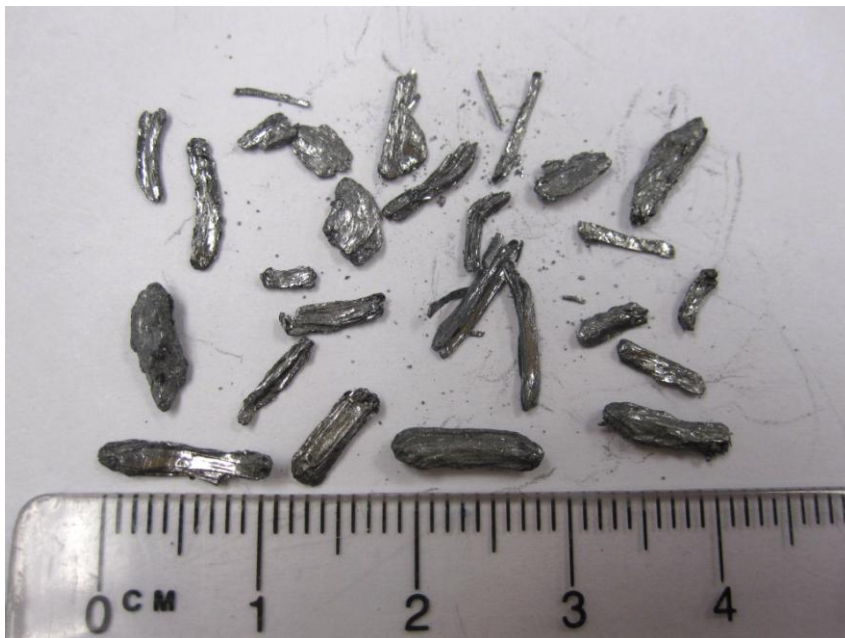
Plate 6. Flake aggregates from RC drill hole WG041 (98-99m)
