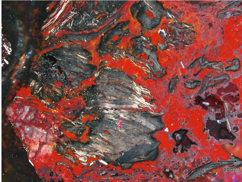
Plate 5. Sample 28718, Hole WG044, 73-74m (PPL), (Xnic). Graphite scattered as individuals and composites, all enclosed within ochreous-red ferruginised ex-felspars and local micas.
