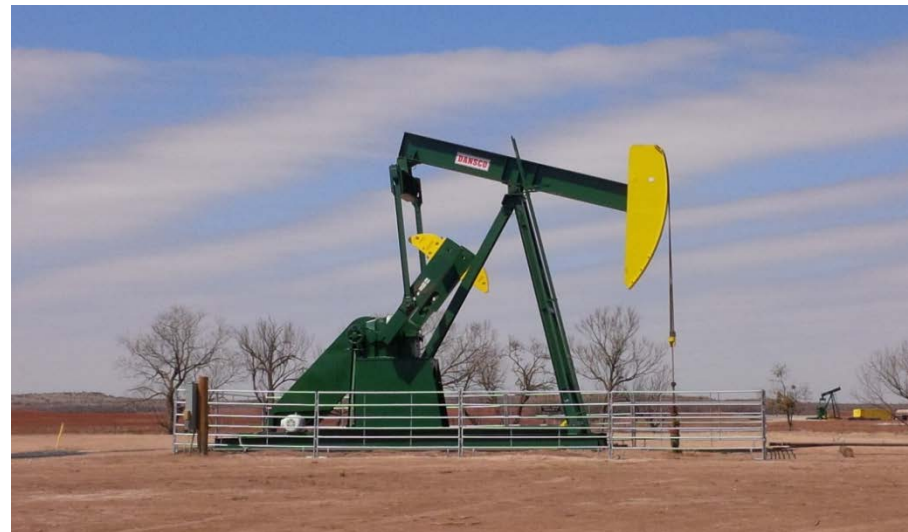
Typical Capitola vertical well lift system
