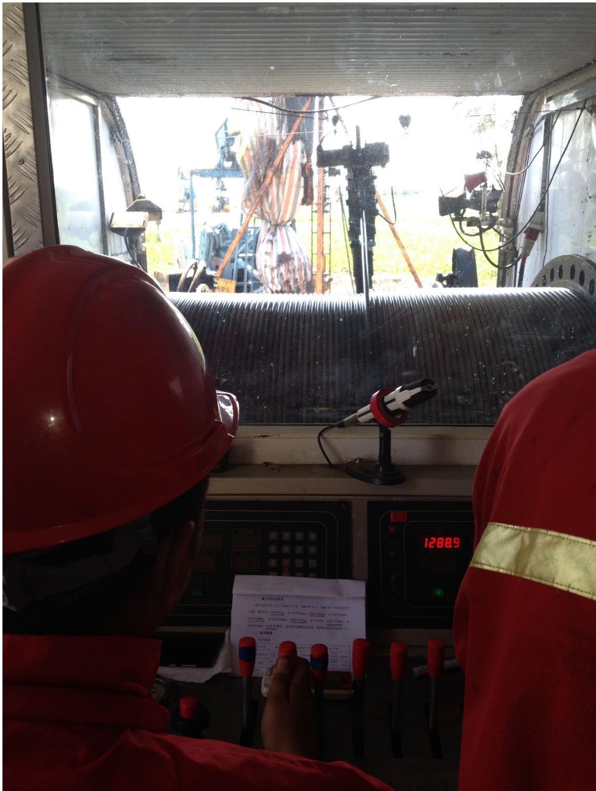
Photo 12 Huaying EOR operator inside the Tubing Truck computerised control room, controls the whole operation over the length of the oil bearing strata deep in the well
