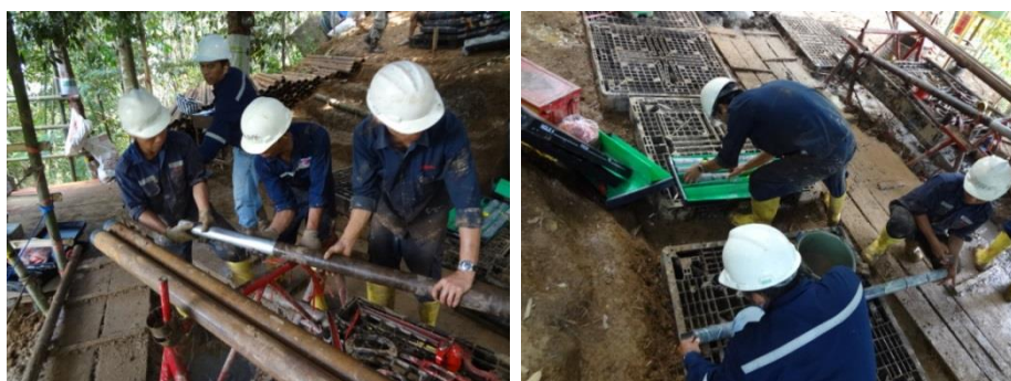
Singgahan Prospect – Maxidrill MXD-420 man-portable rig drilling TRDD058
