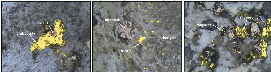
Disseminated chalcopyrite (yellow), bornite (purple grey) & magnetite (light grey) propylitic-potassic altered diorite (TRDD055 & 58)
