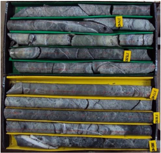
TRDD057 – Quartz-pyrite±chalcopyrite veining in medium-grey, argillic-phyllitic/potassic altered tonalite & volcanoclastic rocks at bottom of hole
