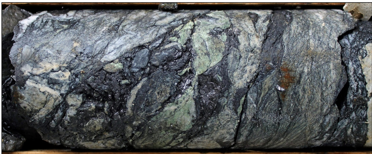
Photograph 5. Close up of graphite deformation breccia mineralization in drill hole GM-21 (104.2m).
