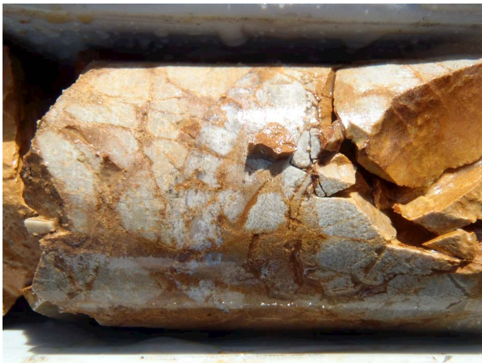
Core, SGRDD039 from 11.3m downhole. Interval 10.7-11.3m, quartz flooded mosaic breccia with limonite staining after sulphides, 4.93 g/t Au (BQ Core 36.40mm diameter)
