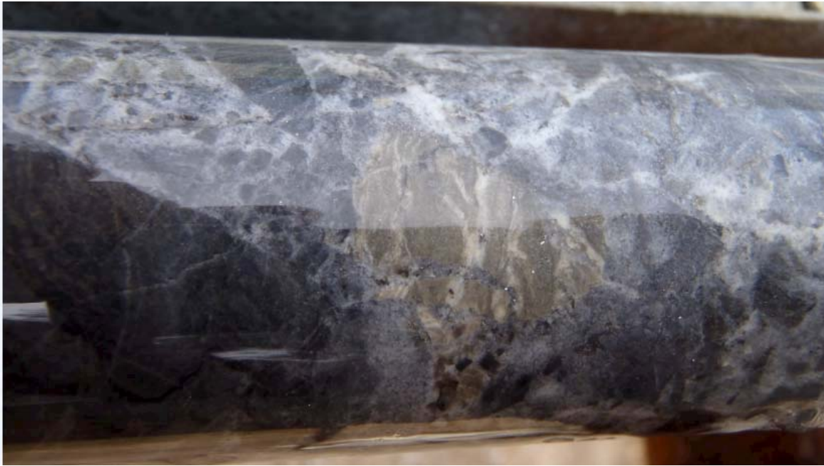
Core, SGRDD43. Brecciated metasediments exhibiting quartz-sulphide-felsic dyke flooding from 32.00-33.00 metres downhole (field of view L-R 70mm). The light brown material in center of the core is a finger of dyke with disseminated sulfides (BQ Core 36.40mm diameter).
