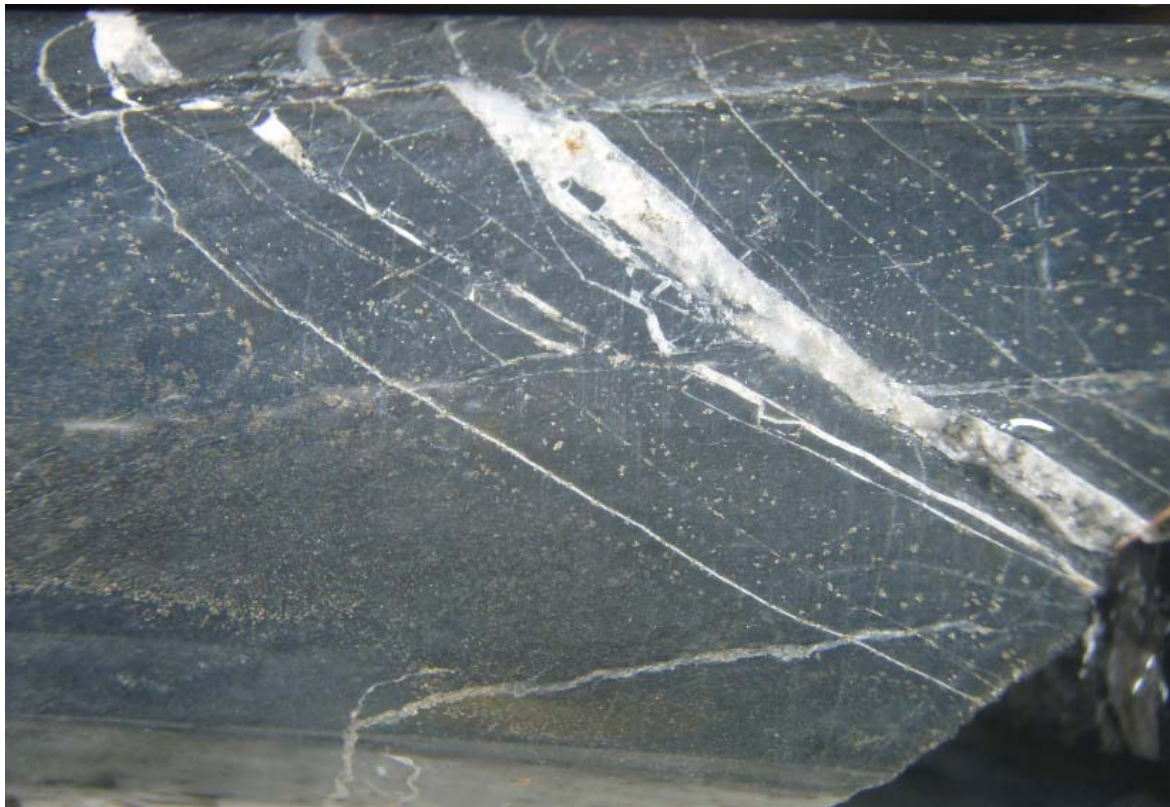
Core, ZK0001. Metasediments with disseminated sulphides and sheeted quartz-sulphide veins from 79.00-80.00 metres (NQ Core 47.60 mm diameter).
