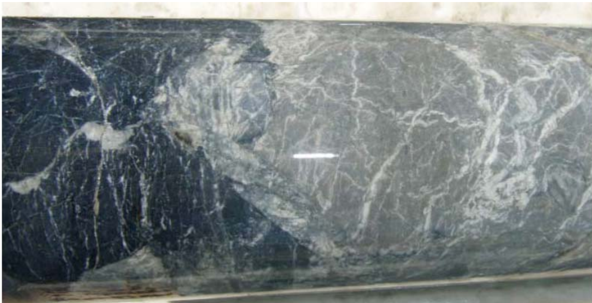
ZK0001 Core from 80.00-81.00m downhole exhibiting alteration and brecciation (NQ Core 47.60 mm diameter). The light grey material is altered felsic dyke material that has carried the mineralising fluids intruding the black metasediments of the Sandon Beds.
