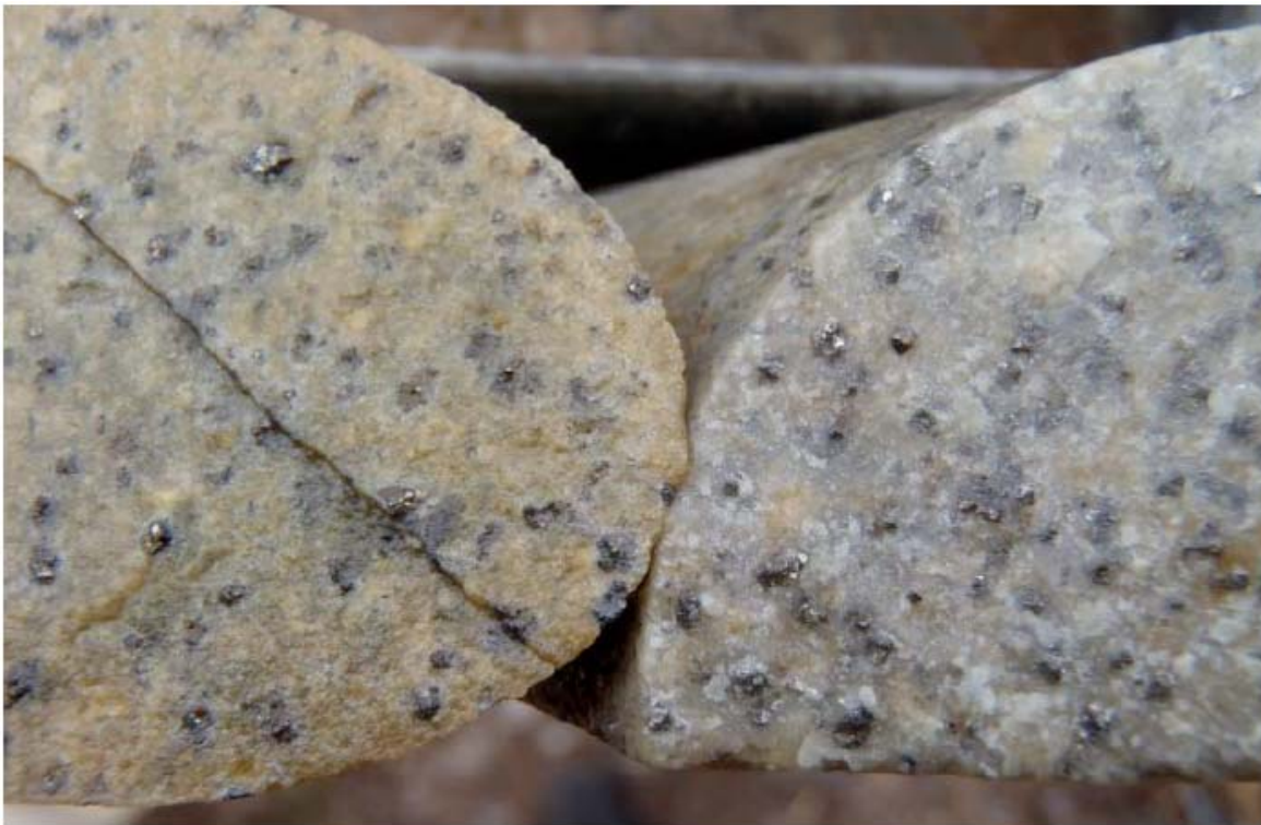
Comparison of core samples altered felsic dyke in SGRDD0043 with SGRDD004 from Martins Shaft. This figure shows the surfaces of sheeted vein alteration in felsic dykes studded with 0.50-2.00mm wide sulphides (field of view L-R 65mm). SGRDD0043 (LHS, 23.40m downhole) and SGRDD004 from Martins Shaft (RHS, 47.45m downhole).
