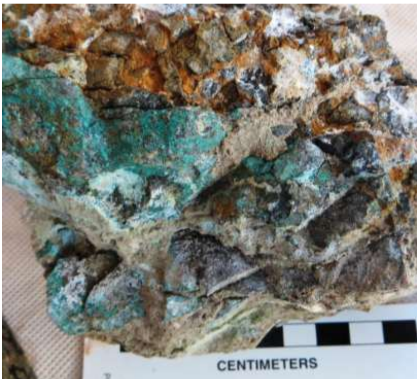
Figure 7: Copper Oxide in brecciated rock sample from Colupo Norte trench.
