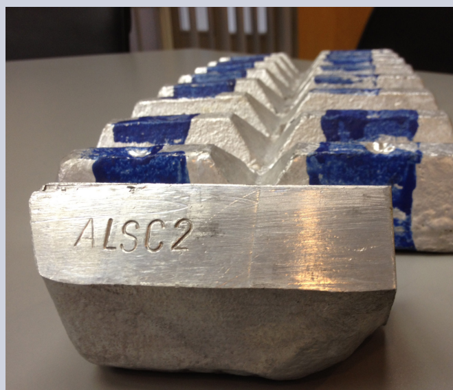
Scandium-Aluminium master alloy waffle ~98% Al & 2% Sc produced by KBM Affilips with whom Metallica has a strategic alliance See ASX Release 7 November and 3 October 2012
