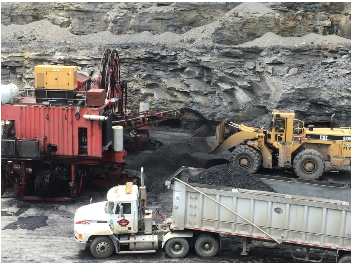
Highwall mining equipment in operation at the Hatfield Gap Mine - Mountainside Coal Company, Kentucky, U.S.
