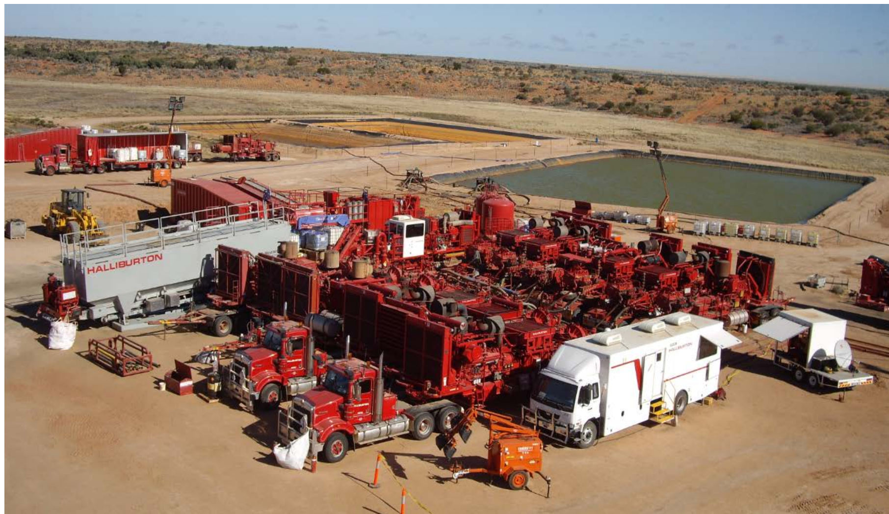
Halliburton high horsepower hydraulic stimulation spread
