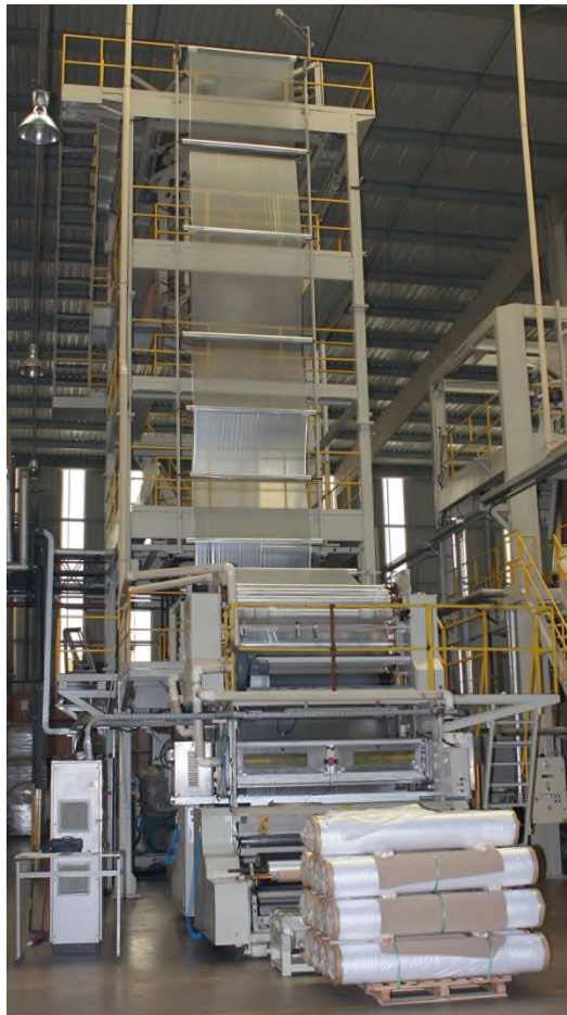
Rulli Standard FE-80 film extrusion line to be set up at Cardia Bioplastics manufacturing plant in Brazil
