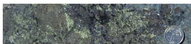
Figure 5: Chalcopyrite-rich zone (yellow) at 129.05m in hole EL14D10.
