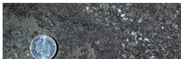
Figure 4: Zinc-rich massive sulphide zone dominated by sphalerite (dark grey), pyrrhotite (bronze), chalcopyrite (yellow) and calcite (very pale grey) at 114.62m in hole EL14D10.
